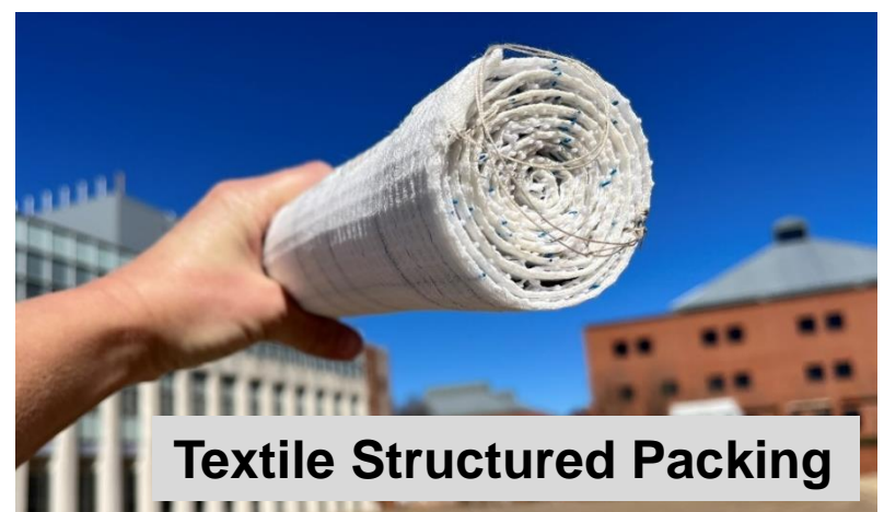
CATSP = Carbonic Anhydrase Textile Structured Packing
