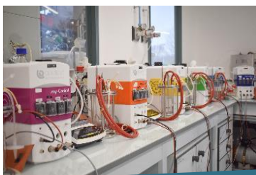
6 x 1L and 2 x 3L Lab-scale bioreactors
