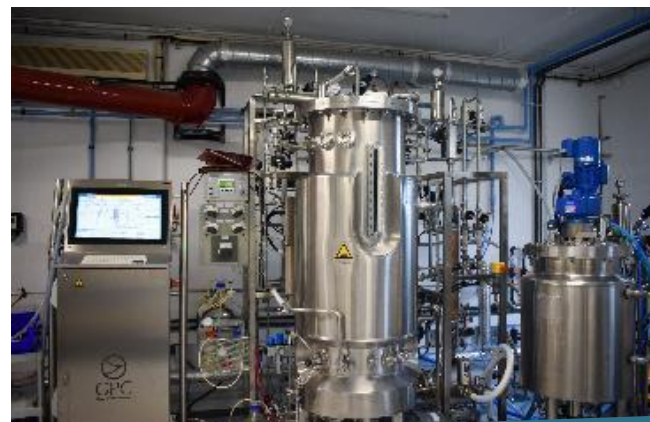
1 x 300L Pilot-scale & Manufacturing fermenter
