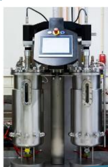
1 x 20L & 1 x 30L Photobioreactors
