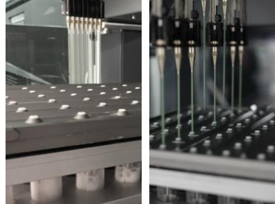
2mag BioREACTOR 48 - 48 HT cultivations (10 mL)
