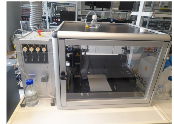
Fig 1 3D printing technology for production of chip substrates, as well as automation for handling of metallic fluids. INBM TUB Freiberg Germany
